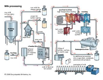
Fat particles are made into a uniform size and resuspended in the milk mixture at different concentrations for different types of milk
