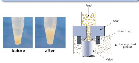
One liquid is made into very small droplets that are re-suspended into the other liquid
